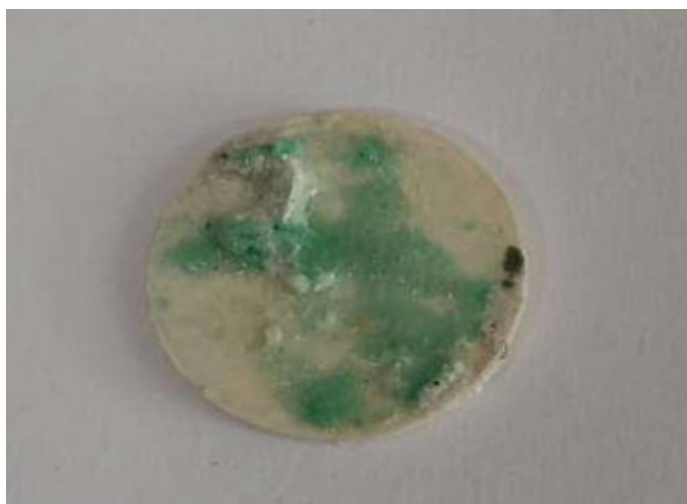
Figure 6. Showing complexation of \text{Ni}^{2+} on the surface of the S2 membrane.
