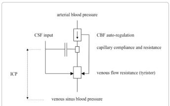
**Figure 3:** Equivalent electronic diagram of the present theoretical model for the relationship between ICP and brain volume decrease.
