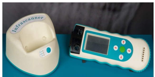
Figure 1: “Near Infrared (NIR) system for detection of brain hematomas, invented by Dr. Britton Chance (University of Pennsylvania) and Dr. Claudia Robertson (Baylor College of Medicine) and manufactured by InfraScan, Inc. The device is a notable advancement in combat casualty care as a triage tool for one of the most problematic diagnoses on the battlefield: traumatic brain injury with intracranial bleeding”. The quote is from the display at the National Museum of Health and Medicine.
