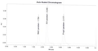
Fig. 1 Chromatogram of the standard solution for parabens
